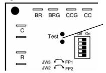
Short test pins together to enter Test Mode and speed-up timing and delays for 20 minutes.
